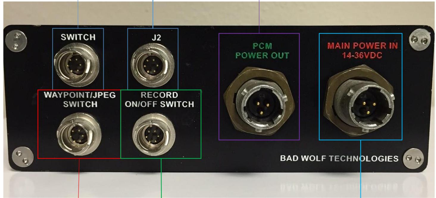
Waypoint/JPEG Switch. Used with GPS or if using JPEG function
